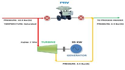
Case : WITH PRV CLOSED & BYE PASS FROM TURBINE
